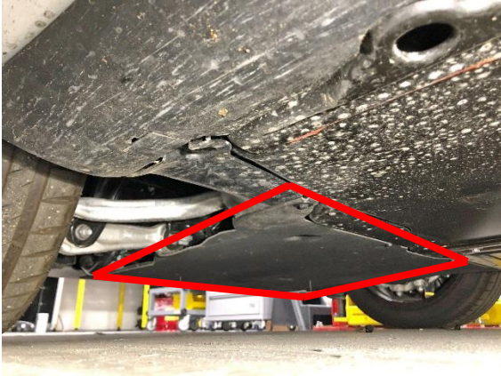
✓ Figure 1 – Front aero shield panel present
